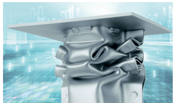
Crack-free buckling during axial crash (welded hollow profile, thickness of 2 mm)
