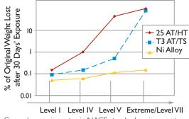
General corrosion rates in NACE standard environments
