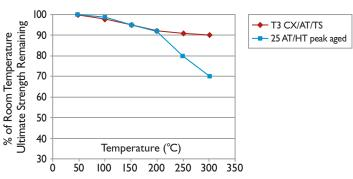
Strength at temperature after 30-minute exposure
