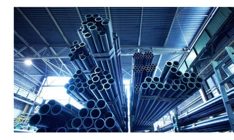
We produce some 40,000 tons of seamless and welded cold-drawn precision steel tubes of up to 17,700 mm in length, with outside diameters from 3 to 180 mm and walls of 0.5 to 22 mm in thickness on state-of-the-art drawing plants at our site in Krieglach (Austria) every year. Our own long-tube production provides the basis for further processing of tubes in the automotive and industrial sector.
