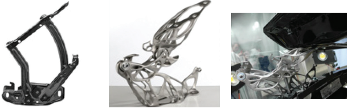
Figure 4 – Engine hood hinge AM redesign: the bionic structure achieved a 50% weight reduction compared to conventional fabrication and enabled integration of a predetermined break point for additional passenger safety
