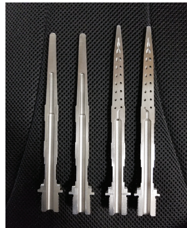
Figure 3 – Core Pins with traditional cooling (top) and conformal cooling (center) with freedom of design afforded by employing AM techniques; section view of each design (bottom)
