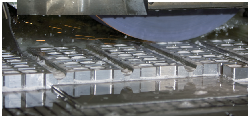
Fine grinding of details in hardened Uddeholm Mirrax ESR
