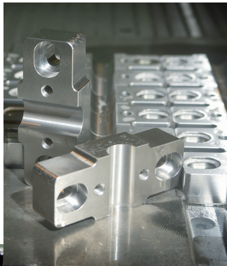
Fine grinding of details in hardened Uddeholm Mirrax ESR
