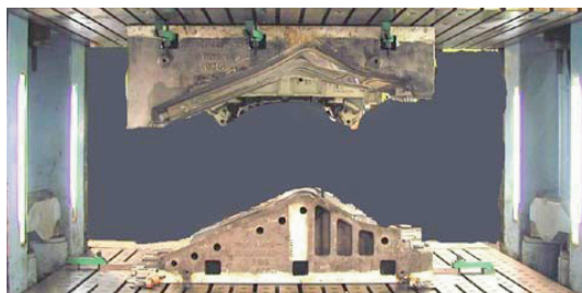
Figure 10. Complex stamping tool.
