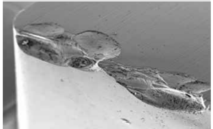
Materials fatigue (chipping)
