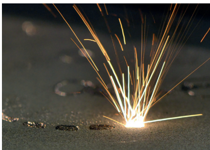
Laser Beam Melting
