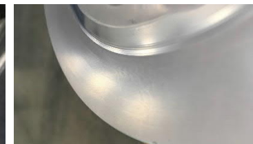
After wet blasting
