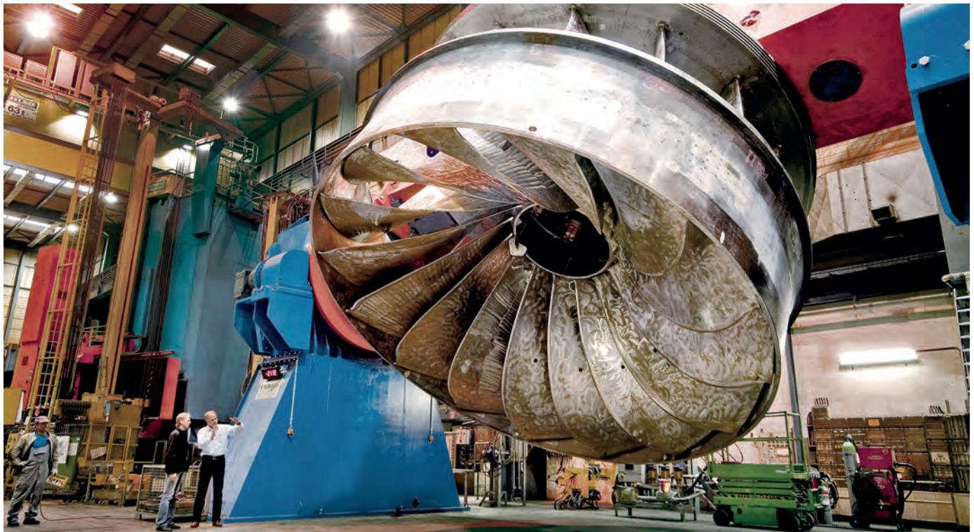
Francis turbine © Andritz
