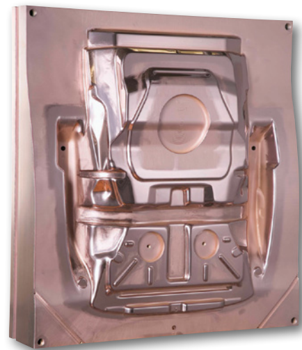
D2 forming die, coated with Duplex-VARIANTIC work material: hot rolled 1.0335 steel.
