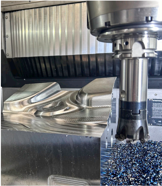
Demonstration segment in pre-machining
