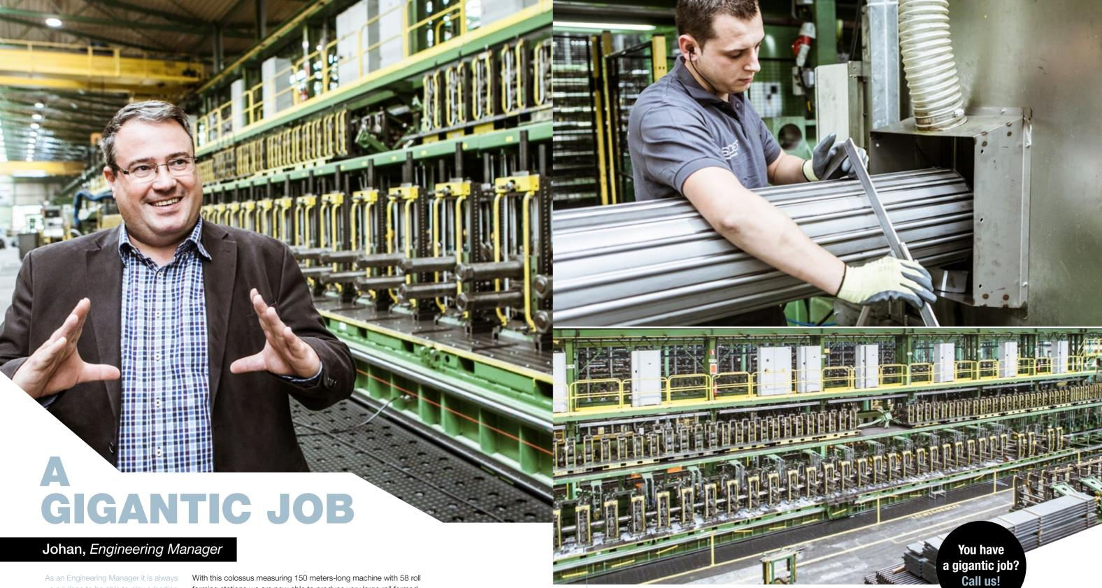
As an Engineering Manager it is always a privilege to be able to play a leading role in the development of our machinery and therefore also that of our company. With this colossus measuring 150 meters-long machine with 58 roll forming stations we are now able to produce very large roll formed tubes with bandwidths up to 1,000 mm and plate thicknesses up to 8 mm - the largest special shaped tubes on the market!
