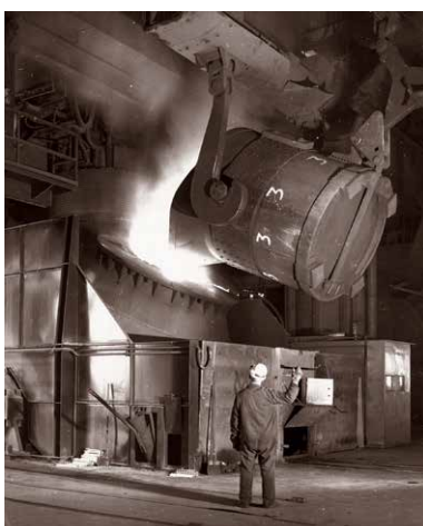
Charging a 50-tonne LD crucible at LD Steelworks 2 in Linz.
