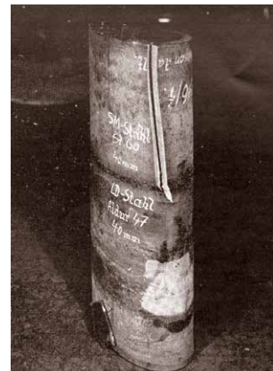
Bending test on a semi-circular tubular element, 1,200 mm diameter, welded from 40-mm gauge LD Aldur 47 structural steel plate (tensile strength 52 kg/mm 2 ) and from St 60 open-hearth sheet steel sensitive to brittle fracture. The sudden fracture occurring during the bending test was absorbed by the LD steel plate close to the weld seam. 51
